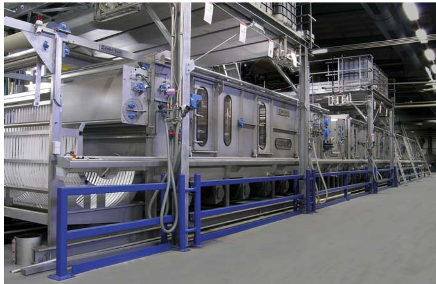
Erbatech's SCOUT pretreatment range PW2/D2 for continuous scouring, pad-steam bleaching and washing of knitwear
