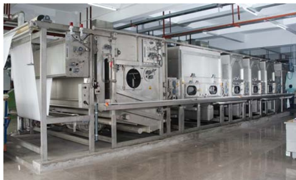
Erbatech's SCOUT TR4/V1 pretreatment range, as installed at Tübas, .....
